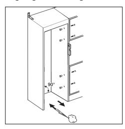
The housing unit must be carefully aligned using a spirit level before installing the appliance. The unit corners must be at right angles, as otherwise the furniture door will not align correctly with the 4 corners of the appliance.
